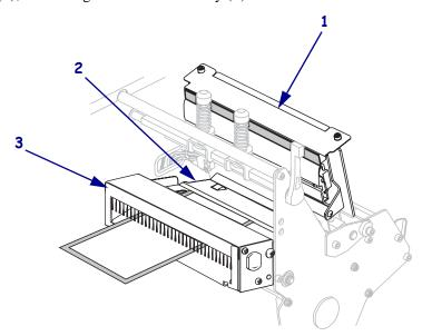
8. Align the media with the inner media guide (1). Slide in the outer media guide (2) until it just touches the edge of the media.
